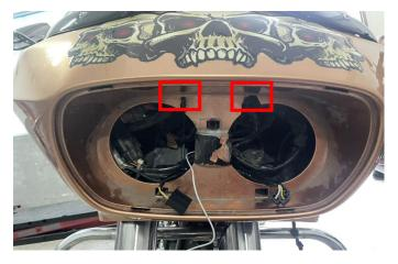
4. Get the ball screws from the original headlight, fix them on the new headlight frame by the fingerprint resistant plate( as the red arrow shown in the picture), connect the wiring harness plug-ins of the headlight and vehicle, start the vehicle, check whether the headlight work normally, and finally, fix the headlight with screws. As shown in the picture:
