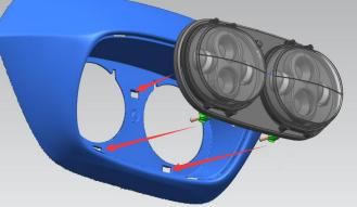
5. After the headlight is installed, clamp the eagle mouth cover (corresponding to the slot during installation). Reinstall the parts removed before, as shown in the picture:
