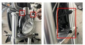
2. Unscrew the screws on both sides of the bracket which fixed the headlights, remove the original headlights, and take out the new headlights. First unscrew the screws on both sides of the new headlights for later use, install the light on the bracket, and then fix it with the screws that just removed, as shown in the picture:
