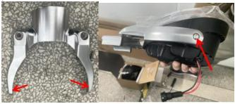
3. Before installing the headlights with the bracket to the vehicle, you need to connect the plugins of the high beam wiring harness and vehicle wiring harness.
