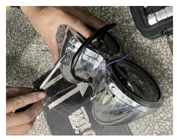
4. Install the new headlamp on the motorcycle, adjust the angle of the headlamp, and then tighten the screws of the mounting bracket. The harness connector of the new headlight needs to be inserted by the owner according to the color sequence in the picture. Connect the plug-in with the overall harness after completion. As the picture shows:
