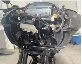
7. Install the crescent-shaped decorative parts(removed just now) on the both sides of the new headlight, and install the headlight on the vehicle(don't tighten the screws)
