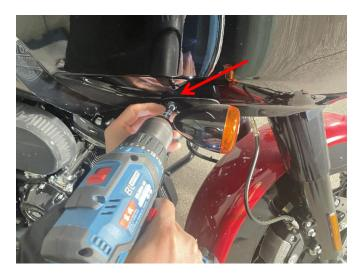
4. Remove the speaker covers on both sides of the front and remove the screws inside the speaker, which hold the front protection cover. Remove the front instrument cover and unplug the wiring harness plug-in of the inside
