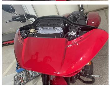
5. Remove the screws that fixed the edge of the front protection cover, and remove the protection cover, as shown in the picture:
