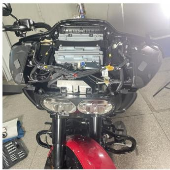
6. Remove the crescent-shaped decorative parts on the both sides of the original headlight, remove the screws that fixed the headlight, disconnect the plug-ins, remove the original headlight, the removed screws for later use. As shown in the picture:
