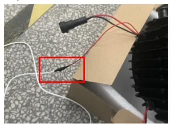
4.Before installing the headlights with the bracket to the vehicle, you need to connect the plugins of the high beam wiring harness and vehicle wiring harness.
