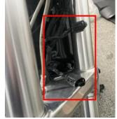
2. Unscrew the screws on both sides of the bracket which fixed the headlights, remove the original headlights, and take out the new headlights. First unscrew the screws on both sides of the new headlights for later use, install the light on the bracket, and then fix it with the screws that just removed, as shown in the picture:
