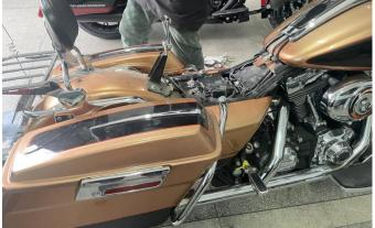
5.Open the lid of the suitcase on one side, unscrew the two rings inside the box, take off the suitcase, and use a tool to pry open the heat insulation decorative board next, as shown in the picture:
