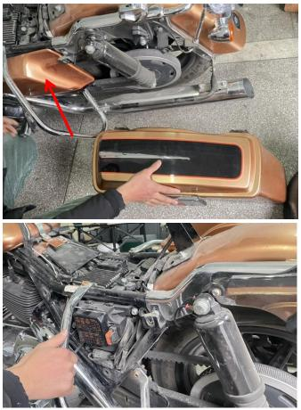
6. Find ACC electrical box, open the lid, use the white extension cord in the accessory bag, peel off the outer skin of one end of the wire, expose the copper wire, connect the electrical box, after connecting, pull it to the headlight place along the fuel tank, as shown in the figure:
