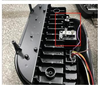
3. Remove the head protection cover, disconnect the harness of the headlamp, and remove the original lamp. As shown:
