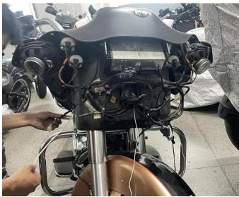
4. Connect the brown and purple turn signal extension wires in the package with the brown wires in the turn signal harness on both sides of the original motorcycle, and then pull the turn signal extension wires on both sides to the headlamp. In the subsequent steps, connect the wire harness with the color corresponding to the new headlight. As shown:
