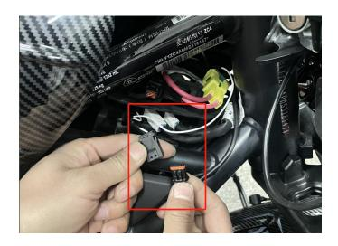
3. After disconnecting the wiring harness of the original motorcycle headlight from the vehicle wiring harness, remove the original headlight. As the picture shows:
