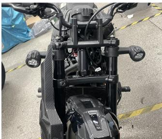
4. Install the original headlight bracket onto the new headlight, then assemble the new headlight onto the motorcycle and secure it with the original motorcycle screws. Then connect the headlight wiring harness to the entire motorcycle wiring harness, and connect the turn signal light wiring harness of the headlight to the turn function wiring harness on both sides respectively. As the picture shows:
