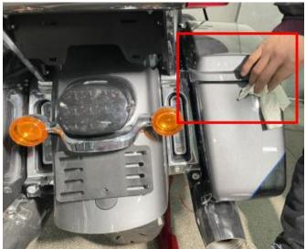
Remove the double-sided adhesive on the back of the taillight, install the light at the edge of the saddlebag opening, press hard to make the lamp fit with the vehicle completely (install the other side as the same steps) as shown in the picture:
