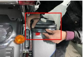
3. Find the original wiring harness that hidden under the rear of the seat cushion and unplug the plug-ins, and reconnect the plug-ins of the original wiring harness with the wiring adapters equipped in the new product, as shown in the picture:
