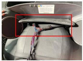
4. Pull the connected adapter cables to the taillights on both sides, connect them with the taillights wiring harness, and sort
