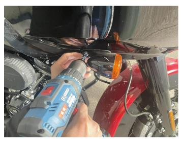
2. Remove the audio covers on both sides of the front of the vehicle, and unscrew the screws inside the audio that secure the front front protective cover. Remove the front instrument cover, disconnect the wiring harness connector of the turn signal inside, unscrew the screws securing the edge of the front front protective cover, and take off the front decorative cover, as shown in the picture:
