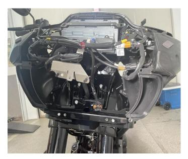
4. Install the decorative lights on both sides on the removed headlights, the wiring harness plug-in on the headlights are connected to the plug-in on the decorative lights, and the plug-in at the other end of the decorative lights are connected with the original vehicle wiring harness plug-in. As shown in the picture:
