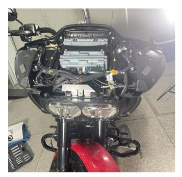
3. Remove the crescent-shaped decorative parts on both sides of the original headlights, unscrew the screws that fix the headlights, disconnect the plug-in, take off the original headlights, and use the removed screws for use, as shown in the picture:
