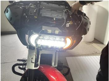
6. After the lights are installed, you can replace the previously disassembled accessories and the front trim cover, as shown in the picture:
