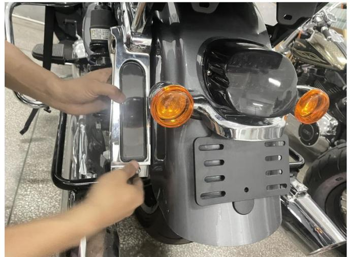
3. Pass the tail light harness through the hole on the mounting bracket, and then use the screws provided in the package to fix it from the back of the mounting bracket (be careful not to tighten the screws too tightly at one time. Tighten the two screws after they are all fixed). The taillight on the other side operate in the same way, as shown in the picture:
