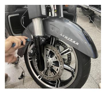
3.Remove the fog light bracket of the motorcycle, disconnect the wiring harness plug-in, and pull the wiring harness of this product to the fog light along the direction of the whole vehicle wiring harness. Connect one end of the wiring harness with steering function to the fog light wiring harness plug-in, and the other end to the vehicle wiring harness plug-in, and finally install the fog light bracket. (The installation steps on the other side are the same as above), as shown in the picture:
