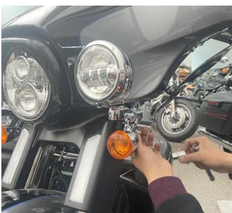
4.Remove the motorcycle headlights and disconnect the wiring harness. Connect the adapter cable provided in the product package with one end to the headlight and the other end to the original car wiring harness; connect the two separate sub-wires to the main wiring harness plug-ins for the brake decorative lights on both sides. Start the motorcycle and turn on the turn signal switch to check if the lamps are functioning properly. Finally put the headlight back in place, as shown in the picture:
