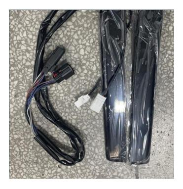
2. Open the saddlebag cover of the original car and remove the cushion. After locating the original car taillight wiring harness plug-in, and disconnect it. Then reconnect it with the corresponding plug-in using the adapter cable provided with the product. As shown in the picture:
