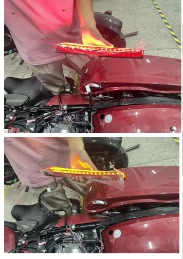
4. Wipe the bottom of the saddlebag of the original car clean with a towel first, then remove the anti-film on the rear shell of the decor light, and stick the decor lights to the bottom of the saddlebag. (The other side can be installed in the same way). Finally, install the original vehicle cushion. As shown in the picture:
