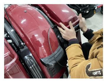
3. Remove the original seat cushion, disconnect the wiring harness plug of the original tail light. used adapter wire in package to ceconnect with the original motorcycle wiring harness plug, and the original tail light wiring harness connected to the adapter wire plug. As the picture shows:
