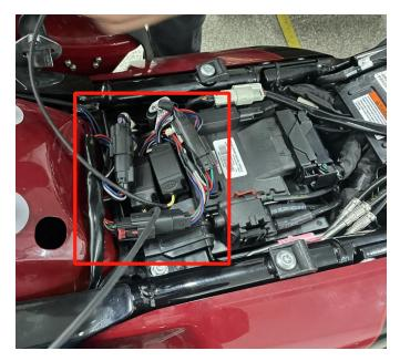
4. Pull the two extension lines on the Adapter cable to the saddlebag tail lamp, connect them with the saddlebag tail lamp harness, and then start the car to turn on the turn signal switch to check whether the left and right turn functions of the saddlebag tail lamp are normal. If there is a function opposite, exchange the connection with the extension line on the other side, and finally install the seat in place. As the picture shows:
