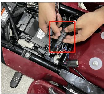
3. Connect the adapter plug in the package to the wiring harness plug in the motorcycle tail
