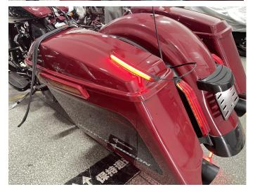
4. Wipe the installation area of the tail light clean, then remove the anti stick film on the tail light, stick the tail light to the edge of the saddlebag cover, and finally press hard to make the tail light better fit. (Please install the tail light on the other side in the same way). Finally, organize the wiring harness and reinstall the original car seat cushion. As the picture shows:
