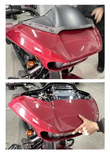
3. First, thread the adapter cable inside the package through the headlight cover, pull it to the windshield position, and connect it to the original motorcycle turn signal plug; Then connect the other end of the adapter cable to the wiring harness connector on the turn signal light (connect the wiring harness in the same way on the other end). After completion, start
