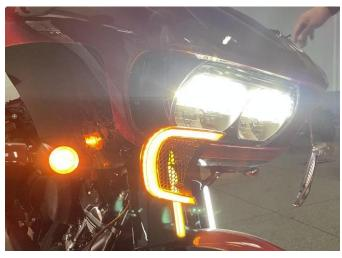
4. Finally, use self tapping screws to fix the turn signal light onto the original headlight frame. As the picture shows:
