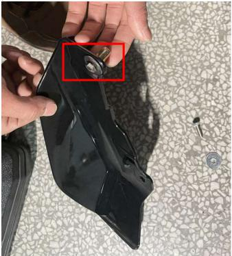
2. In the place where the heat insulation board is installed, install the steel clip in the car body, and then install the heat insulation board and fix it with screws. On the other side, follow the same steps, as shown in the picture:
