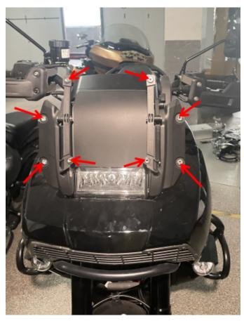
2. Install the new side windshield, distinguish the left and right directions, and then fix them with the original screws, as shown in the picture:
