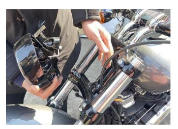
4. Remove the bracket on the back of the original headlight according to the steps in the picture, and replace it with a matching mounting bracket for the fairing.
