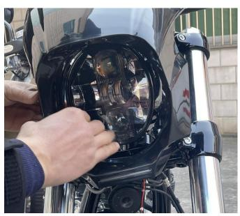
6. Take out the steel clips in the accessories bag, and clip them on both sides of the back of the fairing near the screw holes of the mounting brackets, and then tighten the steel clips through the brackets with screws to fix the fairing (the top of the fairing also needs screws), connect one end of the wire harness plug-in on the fairing to the wire harness plug-in on the original vehicle, and the other end plug-in to the headlight.
