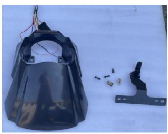
3. Remove the screws securing the original headlights, unplug the headlight harness plug-in, and remove the headlights.
