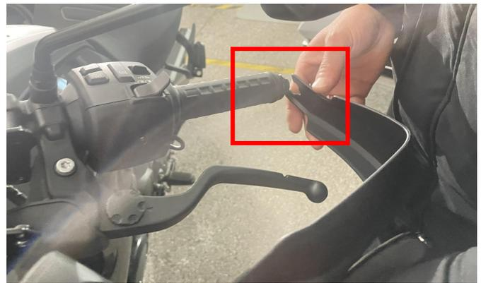
3. First clamp the smoked handguard into the black handguard, then insert one end with the U-notch into the rear of the handguard and fix the other end on the bracket with screws (Install the handguard on the other side by the same steps).
