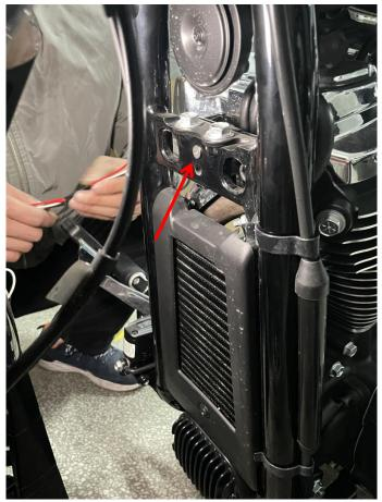
5. Fix the radiator cover on the newly installed bracket with screws. Then connect one end of the harness plug-in on the radiator cover to the harness plug-in of the original headlight and the other end to the integral harness plug-in.
