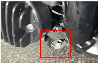
4. Fix the "L" bracket in the accessories package on the inner side of the beam bracket at the top of the original radiator (behind the arrow).
