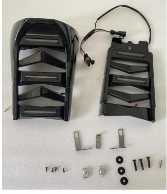
2. Assemble the separate radiator covers together and connect the harness.
