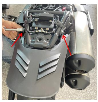
3. After the fenders are installed, put the tail trim cover and seat cushion that were removed before back on the original motorcycle, as shown in the picture:
