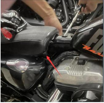
2. First, distinguish whether the product is left or right. Then, peel off the release film on the back of the product. Lastly, use the unscrewed original vehicle screws to pass through the mounting holes of the heat shield and fix it back to the car (The other side is installed in the same way). Shows as the picture:
