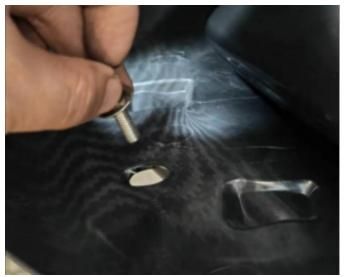
4. Use M6\*16 socket head cap screws and M6 spacers to fix the rear case. As shown:
