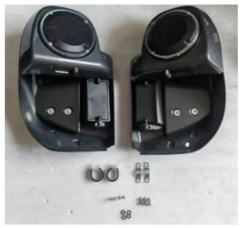
2. Remove the speaker frame with a Phillips screwdriver, keep 8 self-tapping screws and spacers for spare. As shown:
