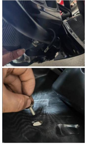
5. Use M6\*16 socket head cap screws and M6 spacers to fix the rear case. As shown:
