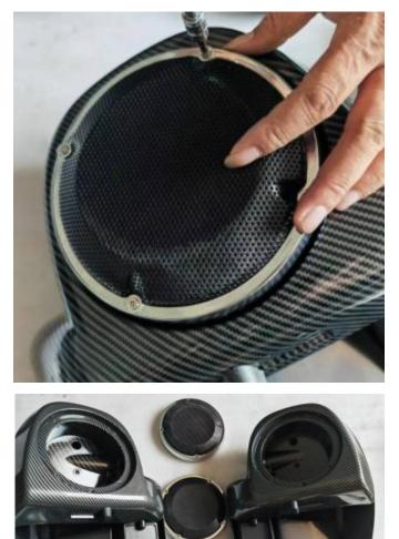
3. Remove the M6\*16 hexagon socket head cap screws and M6 spacers that fix the rear case, and keep the screws and spacers for spare.
