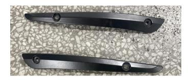
2. Remove the original windshield trim and windscreen of the motorcycle. Than, install the new trim and fix it with original screws (Do not tighten the screws first, and keep a little gap). As the picture shows:
