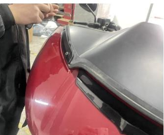
3. Insert the motorcycle original windscreen into the reserved gap, and then tighten the screws. As the picture shows:
