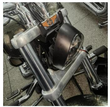
4. Finally, fix the headlight fairing onto the mounting bracket with screws. As the picture shows:
