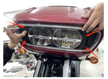
4. Make sure there is no error and then use the matching self-tapping screws to fix the light on the fairing, and finally install the windshield and other accessories back. As the picture shows:
