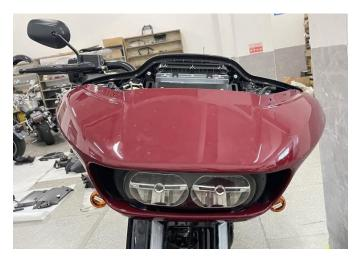
3. Pull the wiring harness of the fairing cover lights from the headlights through the fairing to the windshield, and connect it with the wiring harness plug-in reserved for the original motorcycle, and then start the motorcycle to check whether the light work normally. As the picture shows:
