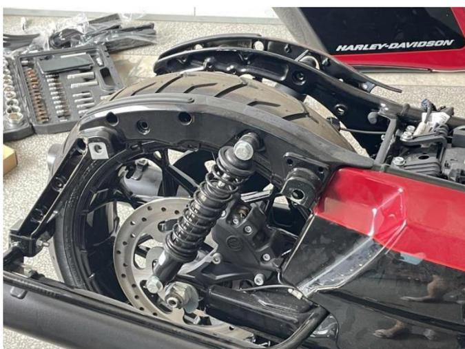
3. Remove the license plate and turn signal bracket from the overall fender. As shown:
