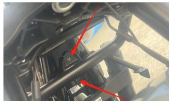
4. Install the left and right ends of the iron bracket A (refer to the product display diagram) in the position as shown in the picture with 2 British M6\*25 hexagon socket head cap screws and 2 M6 flat washers:
