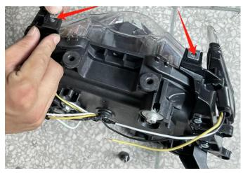
3. Remove the decorative bracket and baffle. and also move to the new headlight according
