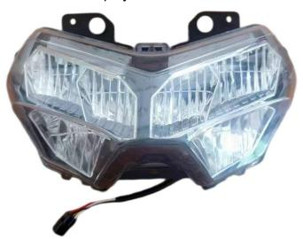
2. Remove the original headlight and decorative cover, then remove the rubber plugs, plugs, steel clips, and small lights on both sides of the original headlight, and move them to the new headlight according to their original positions. As the picture shows:
