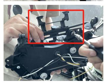
4. After completing the above steps, start installing the headlights. First connect the main harness of the headlights and the daytime running light harness, then start the motorcycle and turn on the headlight switch to check the headlight function. After confirming that there
