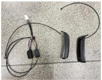
2. Clean the installation position first before install, then distinguish the left lights and right lights sides. tear off the tail lights rear shall's glue film and stick the tail light onto the side saddlebag(which can be installed along the edge of the side saddlebag cover opening), and press firmly to make it better fit. As the picture shows:
