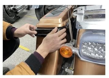
3. Remove the original seat cushion, disconnect the wiring harness plug of the original tail light. used adapter wire in package to ceconnect with the original motorcycle wiring harness plug, and the original tail light wiring harness connected to the adapter wire plug. As the picture shows:
