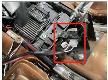
4. Pull the two extension lines on the Adapter cable to the saddlebag tail lamp, connect them with the saddlebag tail lamp harness, and then start the car to turn on the turn signal switch to check whether the left and right turn functions of the saddlebag tail lamp are normal. If there is a function opposite, exchange the connection
