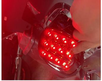
4. Tidy up the connected adapter wires, then fix the taillight.
