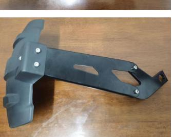
2. Remove the snap ring ,Then remove the screws on the right side of the rear wheel with a wrench as shown in the figue.
