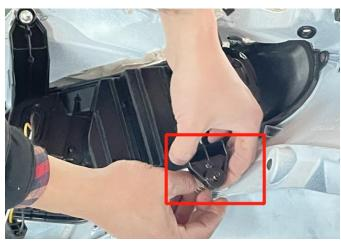
4. Remove the original motorcycle headlamp and replace it with a new one. (Use the original screws for fixing, and each fixing point needs to be using equipped with the spring of the new headlight). As the picture shows:
