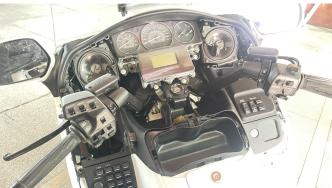
3. Remove the front windshield of the original motorcycle and the headlight mounting cover. As the picture shows:
