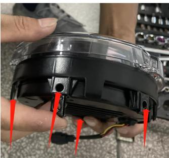
3. Firstly, connect the wiring harness plug of the new headlight to the wiring harness plug of the motorcycle, then start the motorcycle and turn on the headlight switch to check if the headlights are on; After confirming the accuracy, use the original motorcycle screws to fix the
