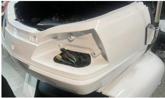
3. Break the green, red green power cords skin of the entire motorcycle tail lamp black connector harness and white brown power cord of the white connector. Then connect the new tail lamp extension cord with them and wrap it with insulating tape
