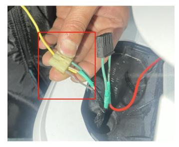
4. Connect the connected extension cable to the same color harness on the new tail lamp, and then start the motorcycle and gently brake. Check the tail lamp function for proper operation. After confirming that there is no error, perform fixed installation (the other side is replaced and installed in the same way)
