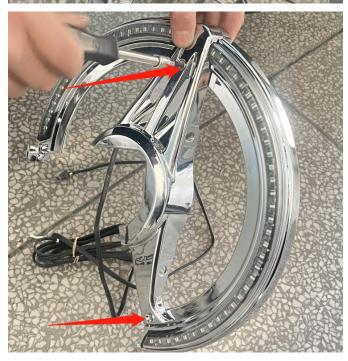
5. First install the L-shaped bracket on the top of the decorative light (note: the screw holes on the L-shaped bracket need to be aligned with the screw holes on the motorcycle's upper fender), and then install the decorative light on the motorcycle. Finally, fix it with screws. As the picture shows:
