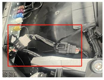
7. Pull the wiring harness on the decorative light along the gap of the motorcycle to the seat cushion, and connect it with the reserved plug-in on the adapter line. (The decorative light on the other side can be installed according to the above steps.) After the decorative light on the other side is installed, the mudguard and seat cushion can be installed back in place. As the picture shows:
