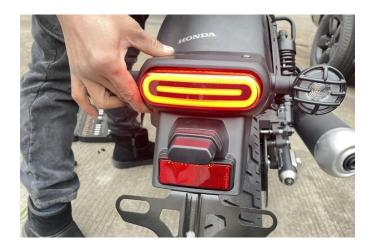
6. Place the wiring harness of the new tail light along the seat cushion in the same way as the original motorcycle wiring harness, reconnect the power plug, then install the outer frame of the tail light back onto the motorcycle, and finally fix the cover of the mudguard and the rear shelf. As the picture shows:
