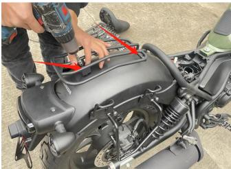
3. Pry out the fixing clip on the cover of the mudguard, separate the cover from the mudguard (to facilitate the subsequent tail light wiring harness), and then remove the original tail light outer frame. As the picture shows:
