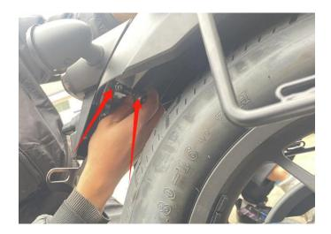
4. Remove the original license plate bracket and the original tail light (disconnect the original tail light harness connector in advance). As the picture shows:
