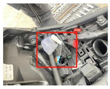
5. Replace and install a new tail light (when installing the tail light, the water leakage port should be installed downwards). First, connect the tail light harness plug to the original motorcycle, start the motorcycle to check the tail light function, confirm it, and then fix it with screws. Finally, install the license plate bracket back in place. As the picture shows:
