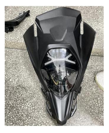
4. Connect the wiring harness connector on the new headlight to the original motorcycle connector, and then turn on the headlight switch to check if the headlight lights up normally. After confirmation, install the headlight and decorative cover back onto the original motorcycle, and finally reinstall other decorative components. As the picture shows:
