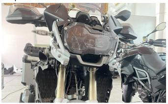
3. Fix the auxiliary lamp bracket onto the original motorcycle using the screws and nuts provided with the product, and then reinstall the headlight decorative cover. As the picture shows:
