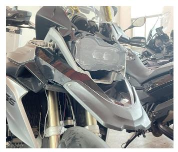
5.Fix the lighting lamp to both ends of the auxiliary lamp bracket using matching screws and nuts. As the picture shows:
