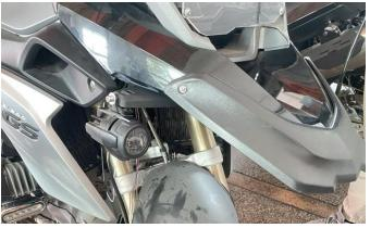
6.First, fix the control switch to the original handle using the original screws, and then pull the wiring harness in the package through the gaps to the front auxiliary light and the original motorcycle battery. Finally, connect one end of the wiring harness to the auxiliary lamp wiring harness, and the other end to the positive and negative poles of the battery. As the picture shows:
