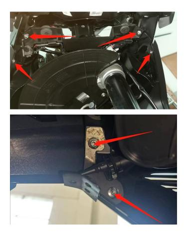
3. Prepare the installation bracket for the auxiliary light, secure it to the small bracket in step 1 with screws, and then install the auxiliary light at both ends of the bracket. As the picture shows:
