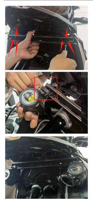
4. First, use the original screws to fix the control switch to the original handle. Then remove the seat cushion and the exterior decoration of the fuel tank. Afterwards, Pull the end of the connecting wire harness with a port
