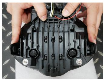
9.Use a 9/32 socket to remove the bracket at the red circle position and remove the I-shaped wire plug and liner for later backup. As the picture shows:
