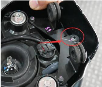
5.Remove the screw indicated by the arrow and separate the headlight frame from the headlight. As the picture shows:
