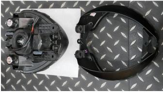
6.Remove the rubber plugs on both sides of the motorcycle lights for later use. As the picture shows:
