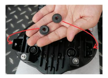
8.Effect image after installing the rubber stopper. As the picture shows:
