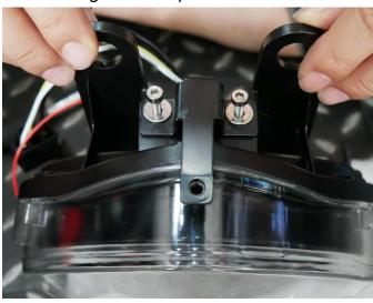
11.Install the outer frame removed in step 5 onto the new LED headlight. And tighten the screws at the red circle position. As the picture shows:
