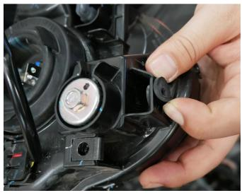
7.Install the removed rubber plugs into the installation holes on both sides of the new LED headlight aluminum rear housing. As the picture shows:
