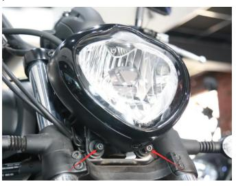
3. Remove the exposed wiring harness (circled in red). Separate the headlight from the wiring harness of the motorcycle. As the picture shows:
