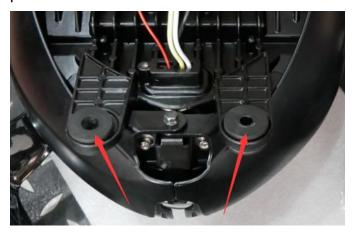
13.Install the headlight decorative frame removed in step 4 onto the new LED headlight and tighten the screws. As the picture shows:
