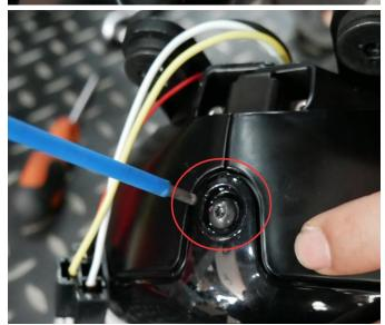
14.Install the new LED headlight with the headlight decorative frame onto the motorcycle and connect the headlight wiring harness. As the picture shows:
