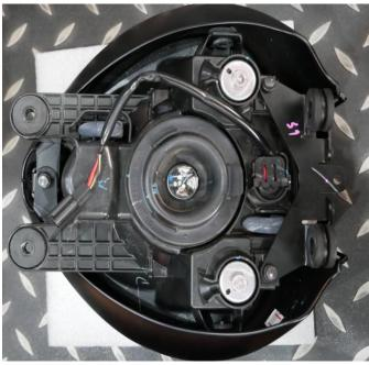
4. Use a 3mm Hex key and cross screwdriver to unscrew the screw pointed by the red arrow. Remove the headlight decorative frame for
