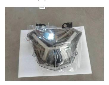
2. First, remove the original windshield, headlight decorative cover, and headlights. The circular rubber pads and steel clips on the original headlights should be moved to the new headlights according to their original positions. As the picture shows:
