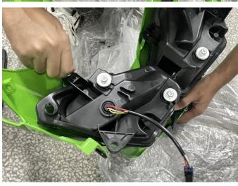
4. Install the installed headlights and headlight covers back onto the motorcycle and connect the wiring harness connectors. Then start the motorcycle, turn on the headlight switch, and check if the headlights are working correctly. After confirming the accuracy, install the seat cushion and decorative panels on both sides back onto the motorcycle. As the picture shows:
