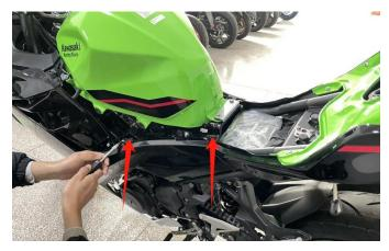
3. Remove the original rear seat exterior trim parts and license plate bracket of the motorcycle. As the picture shows:
