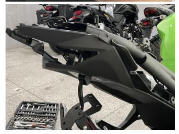
5. First, remove the rubber ring from the original tail light and move it to the new tail light according to its original position. Then, fix the iron bracket in the package to the rear shell of
