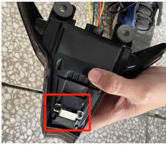
6. Install the new taillights back onto the motorcycle and connect the wiring harness connectors. Then connect the tail turn signal
