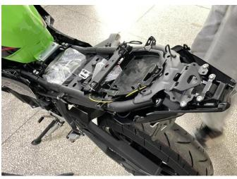
4. Remove the original motorcycle tail light bracket (if no have, can be omitted) and tail light, then disconnect the tail light harness connector.
