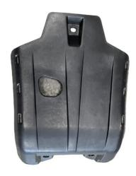
2. First, remove the bracket under the original motorcycle engine, and then install the skid plate under the engine and fix it with the matching screws. As the picture shows:
