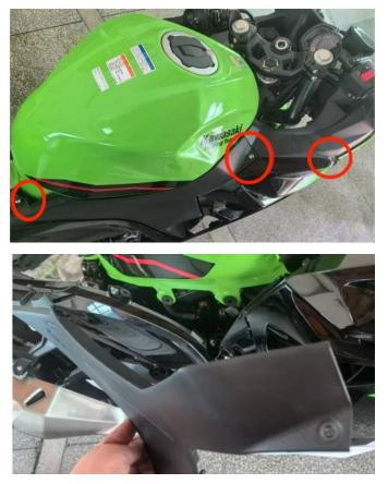
4. Thirdly, remove the following accessories sequentially and keep them for later use: 3 screws and 1 plastic buckle in picture ①, 1 screw in picture ②, 4 plastic buckles in picture ③, 2 screws in picture ④, 1 screw in picture ⑤, and then remove the plastic side panels part. As the picture shows:
