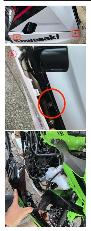
5. Fourth, remove the iron bracket of the original bike, and install the bracket R on the frame with the two screws removed; Then remove the ball screws of the original bike, and install the bracket A with the outer hexagon screws of M10\*90. As the picture shows.
