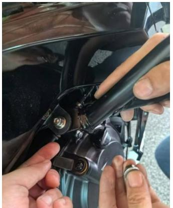
8. Finally, fix the lower right end of the engine guard bar on bracket A with the hexagon screw of M12\*20. Tighten all the screws together.
