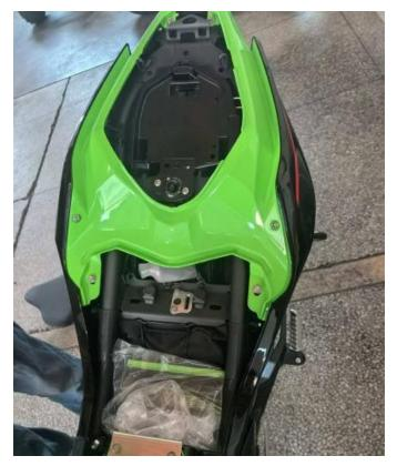
3. Secondly, remove and keep the three original screws, then remove the plastic side panels. As the picture shows:
