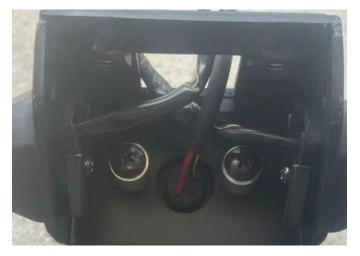
6. Secure the license plate mounting bracket to the rear frame with the four screws removed from the motorcycle, and restore the wiring harness to its original state. As the picture shows:
