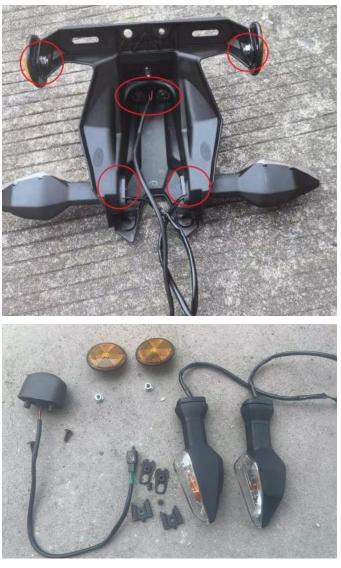
5. Mount the 3 lights to the iron license plate mounting bracket and add 2 aluminum post assemblies to the location light place. As the picture shows:
